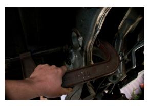
DO NOT TORCH THE OEM BUSHING! Applying heat can alter the temper characteristics of the aluminum subframe and significantly weaken it. This applies to 350Z only, all 370Z including Nismo editions have steel subframes.
