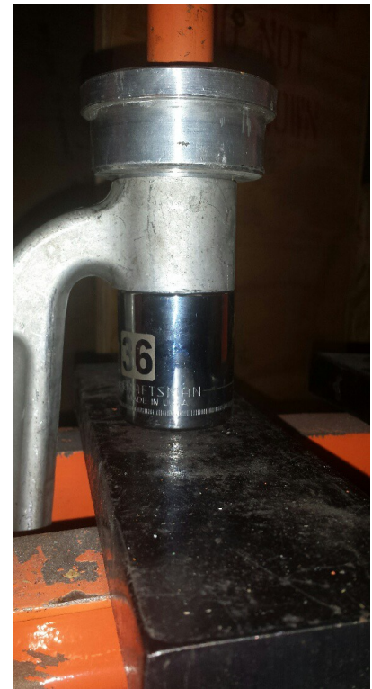
SPL diff bushing driver on top, 36mm socket as receiver on bottom.
