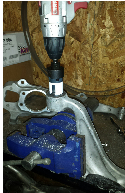
Proper alignment of hole saw.
